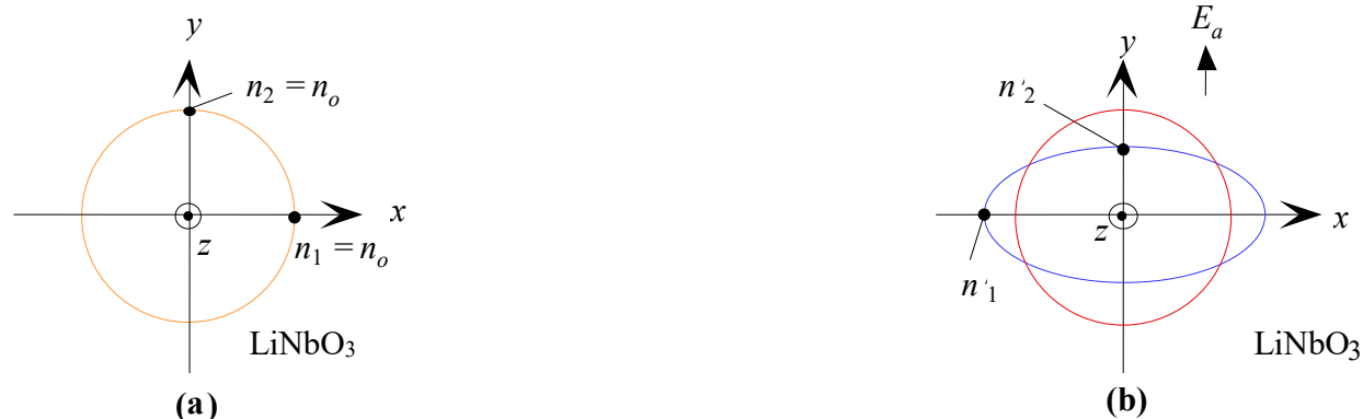
Figure: (a) Cross section of the optical indicatrix with no applied field, n_1 = n_2 = n_o (b) Applied field along y in LiNbO 3 modifies the indicatrix and changes n_1 and n_2 change to n'_1 and n'_2 .
